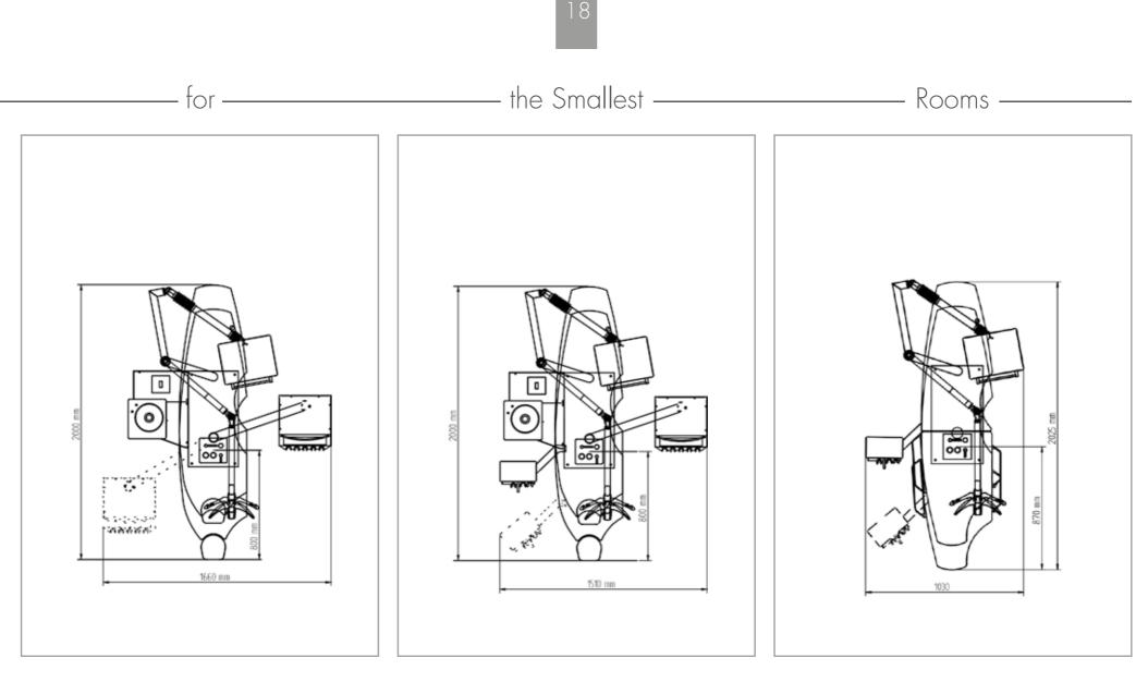
Dimension sheet for the L1-ECO AIR, L1-ECO and L1-S300 models. The doctor's device with integrated suction tubes can be swivelled to the doctor's or the assistant's side. Lowest position: 570 mm Highest position: 800 mm Dimension sheet for the **L1-S600**, **L1-ECO** and **L1-ECO-AIR** models with an assistant's device. Lowest position: 570 mm Highest position: 800 mm
