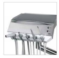
With the **L1-ECO** model, the instruments are driven via a simple control system. It can be equipped with a 3-function syringe, a turbine connection and a 1,000-40,000 rpm micromotor. The suction tubes are in the doctor's device.
