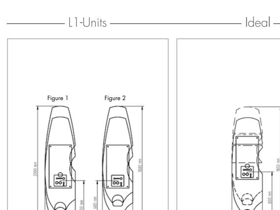
This dimension sheet shows the L1-SOLO model with a long back rest (figure 1) and the L1-SOLO model with a short back rest (figure 2). Lowest position: 570 mm
